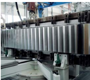
Racks and workpiece holders before hardening treatment.
